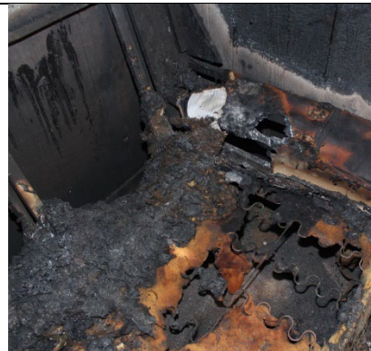
Figure 8 – End of sofa and arm where a small fire was first observed.
